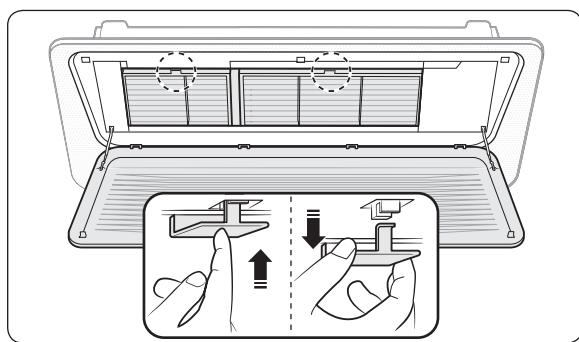
Press the Push signs (▽) on the air filter. Grab the handle of the air filter and pull it out from the indoor unit with your hand.
