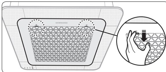
Push down the hooks at each side of the front grille to open the grille.
