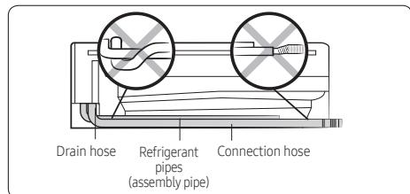
In Step 2-2, step 3 you determined the exit position for the piping bundle. The unit has three knockouts available for the left, right, and bottom exits. When the bundle exits directly from the rear, none of the knockouts are used.
