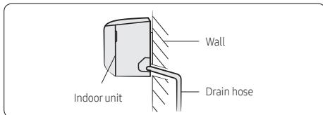
3 Based on the hole location, determine where the piping bundle (drain hose, refrigerant pipes, and cables) will exit the unit.
